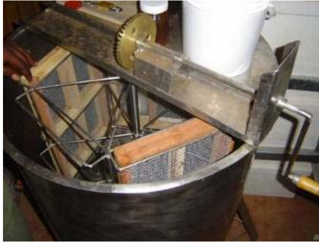
Photograph 32 - a centrifuge which can handle honey from the KTBH (placed in baskets) as well as the Langstroth hive
