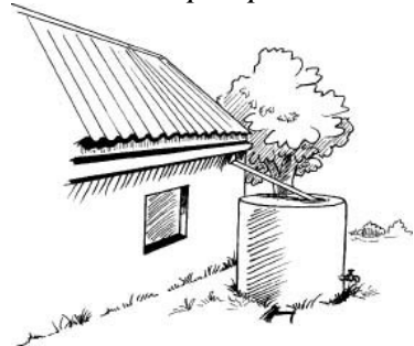
Above-ground tank. This can be used only with a metal roof.
