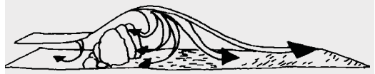
A poorly managed windbreak: The trees block the wind totally. The wind whirls behind the windbreak, it spoils the soil surface and vegetation behind the windbreak.
