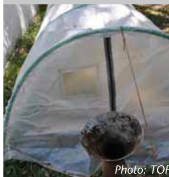
The flexi gas biogas (above) system is housed in a greenhouse to protect it from the sun and prolong its lifespan(below)
