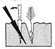
4. Pull handle of planting bar, firming soil at bottom of
